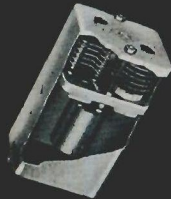
FIXED-TUNED EXCITER TANK
