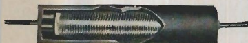
Cross Section — showing progressive interleaved windings for higher resistance values in less space.
